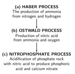
Figure 23.9: Flow diagram showing steps in the production of nitrogen fertilisers
