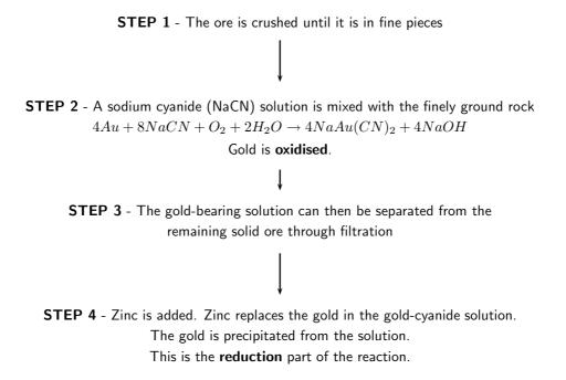
Figure 21.3: Flow diagram showing how gold is processed
