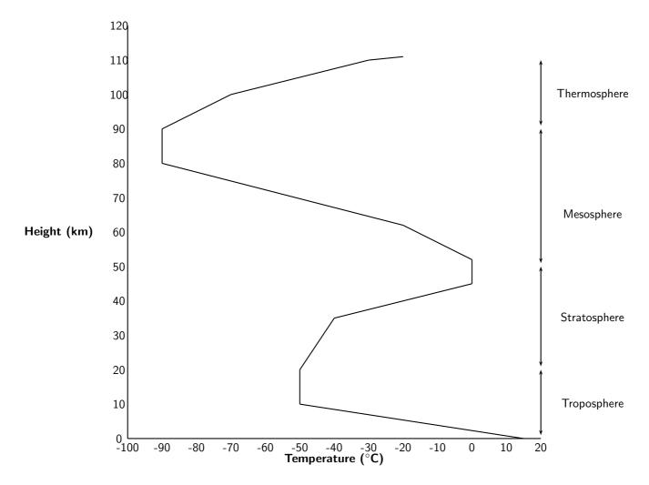
Figure 22.1: A generalised diagram showing the structure of the atmosphere to a height of 110  $\,\rm km$
