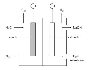
Figure 23.6: Membrane Cell
