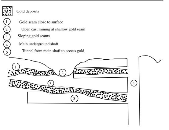
Figure 21.2: Diagram showing open cast and shaft mining
