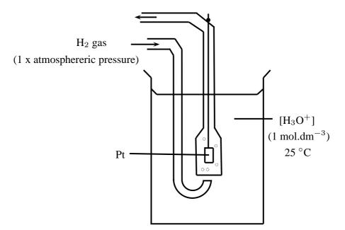
Figure 17.3: The standard hydrogen electrode
