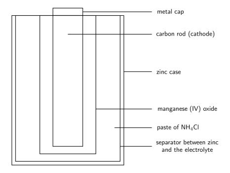
Figure 23.11: A zinc-carbon dry cell
