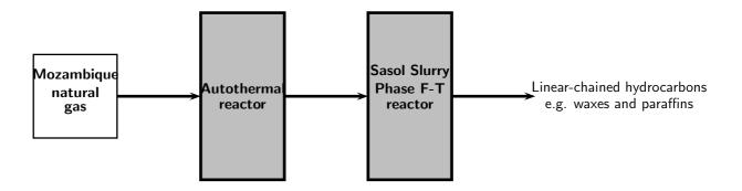
Figure 23.3: Conversion of natural gas to liquid fuels
