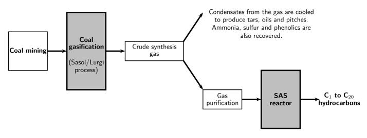
Figure 23.1: The gasification of coal to produce liquid fuels
