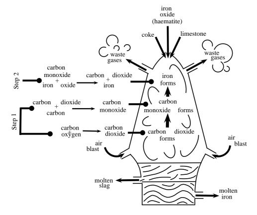
Figure 21.4: A blast furnace, showing the reactions that take place to produce iron
