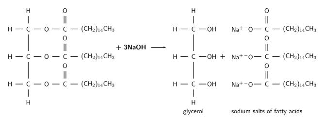
Figure 23.8: Sodium hydroxide reacts with a fat to produce glycerol and sodium salts of the fatty acids
