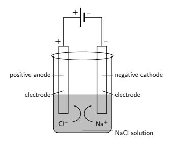
Figure 17.7: The electrolysis of sodium chloride
