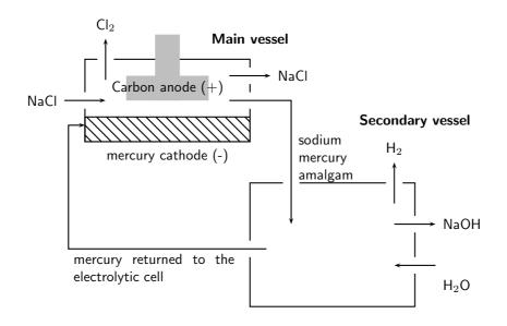
Figure 23.4: The Mercury Cell
