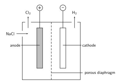
Figure 23.5: Diaphragm Cell
