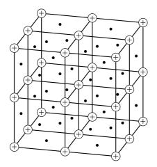
Figure 4.11: Positive atomic nuclei (+) surrounded by delocalised electrons  $(\bullet)$
