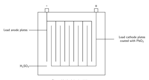
Figure 23.10: A lead-acid battery
